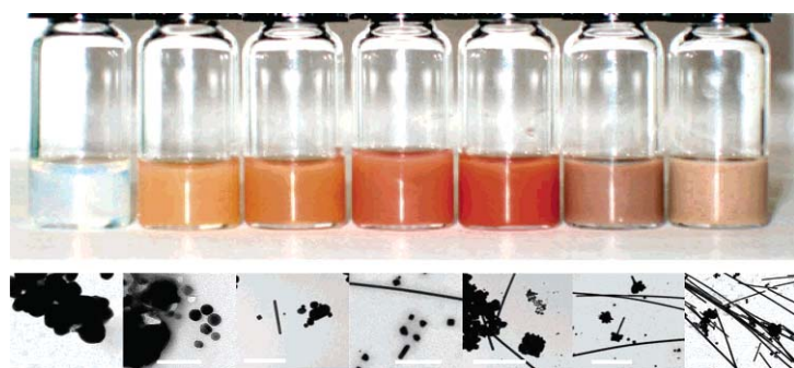
Figure 1 Product of Microwave Assisted Polyol Process as a Function of Heating Time (30 to 210 sec left to right.) Scale bars are 200 nm, 100 nm, 500 nm, 500 nm, 1 mm, 1mm, and 1 mm in lower figures 24 .
