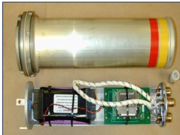
Raytheon RFID Bulk STag for Patriot Missile Health Monitoring Mil Spec Qualified
