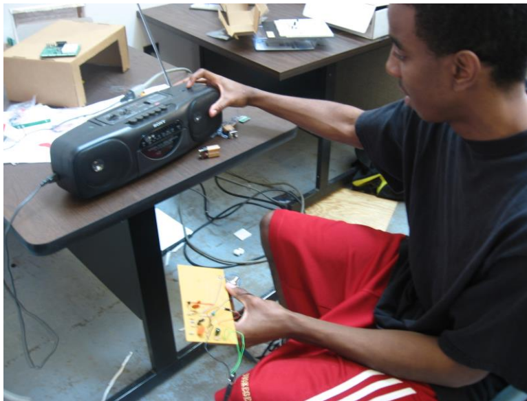
Figure 2: An electrical engineering student at Tuskegee University is trying to pick up signals from his FM transmitter on a radio receiver.
