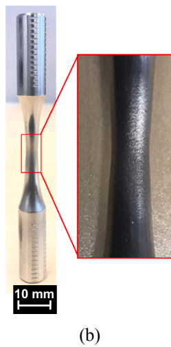
Fig. 11. (a) Stress amplitudes versus fatigue lives obtained under rotating-bending (R-B) and axial loadings for wrought 316L SS specimens, and (b) a wrought 316L SS specimen, which was subjected to stress amplitude of 425 MPa and had a fatigue live, 2N_f = 5,780 reversals. This specimen failed due to excessive deformation at the gage section.
